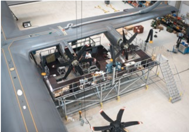
Mobile propeller dock for servicing and maintenance work on a LOCKHEED C-130 HERCULES
