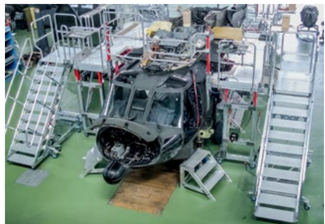
Both of these height-adjustable, contour adaptable work platforms enable optimal maintenance work on a BLACK HAWK
