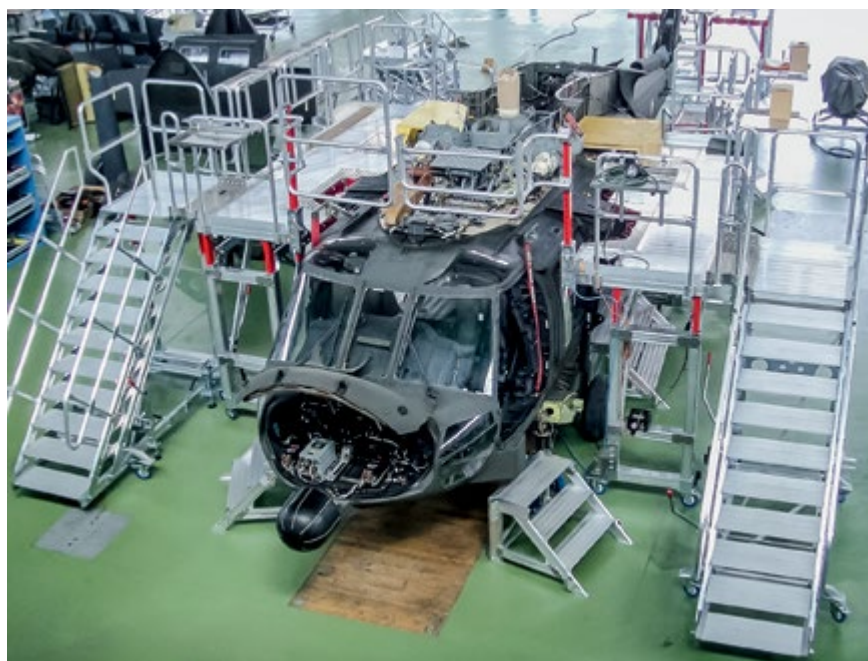
Height-adjustable work platforms with contour adjustment to enable optimal maintenance work
