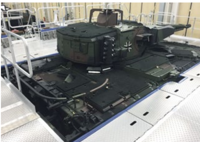
Contour-adapted maintenance platform around a PUMA tank
