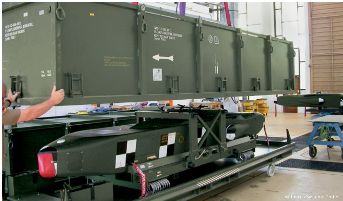
Airtight special container for transporting and storing missiles.
