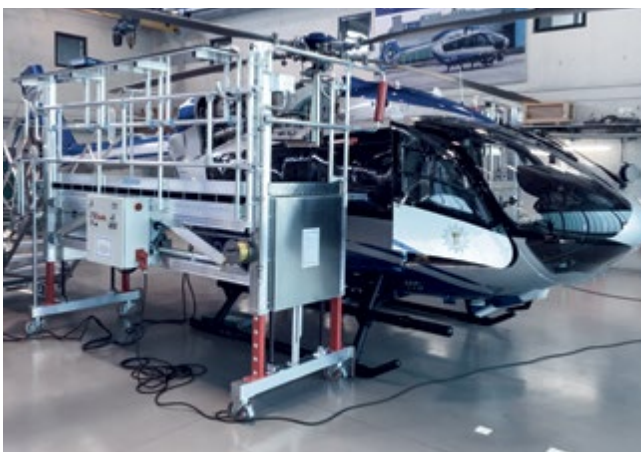
Electric height adjusters and mobile maintenance platform for the H145 police helicopter
