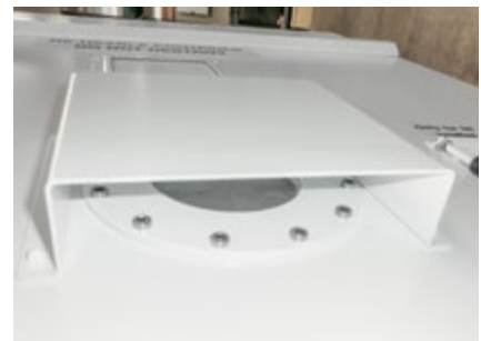
Safety feature Rupture disc: Provides protection in the event of a sudden ambient pressure drop.
