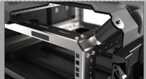
**Wall Mounted Cylindrical shocks.** The shock mounts on V-Rack cases are attached directly to the case wall. They isolate equipment from vibration as well as impact forces. This shock mount design is used for lower payload weight applications.
